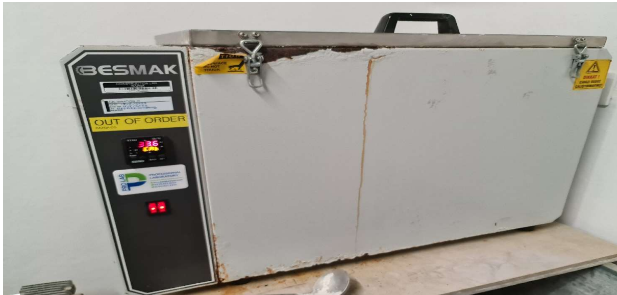
Boiling container Instrument with Digital heat indicator according to the (ISO 10545-3)
