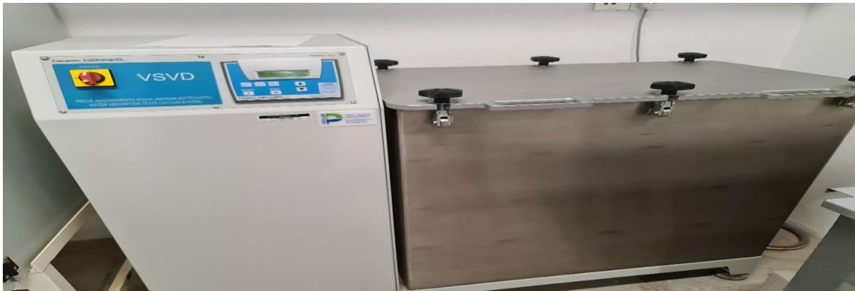
Vacuum Pressure Instrument full automated according to the (ISO 10545-3)
